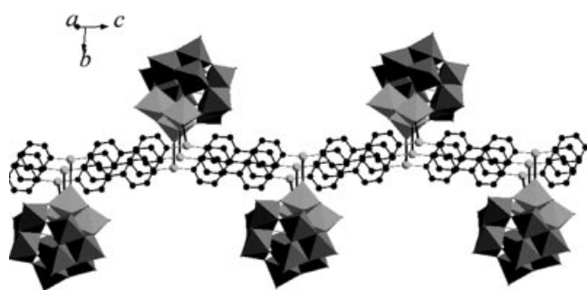
Figure 2. Combined polyhedral/wire representation of the 1D chain structure in 1 . The dark grey polyhedra represent the molybdenum polyhedra and the light grey polyhedra the \text{Mo}_3\text{O}_{13} triad bound to \text{Cu}(\text{bipy}) .
